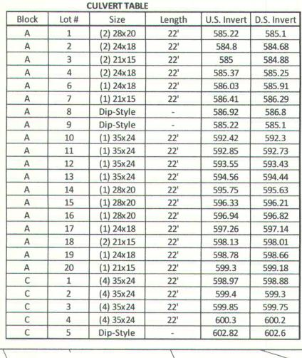
CONTRACTOR SHALL PLACE THE DRIVEWAY CULVERT WITHIN THE EXISTING BAR DITCH FLOWLINE AND PROVIDE A MINIMUM OF 1% SLOPE FOR POSITIVE DRAINAGE AND A MINIMUM LENGTH OF 22 FEET PER WILLIAMSON COUNTY REQUIREMENTS. **EXACT DRIVEWAY LOCATIONS MAY**
