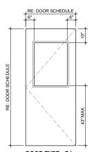
DOOR TYPE - D1 NEW, FLUSH, SOLID CORE, WOOD DOOR
