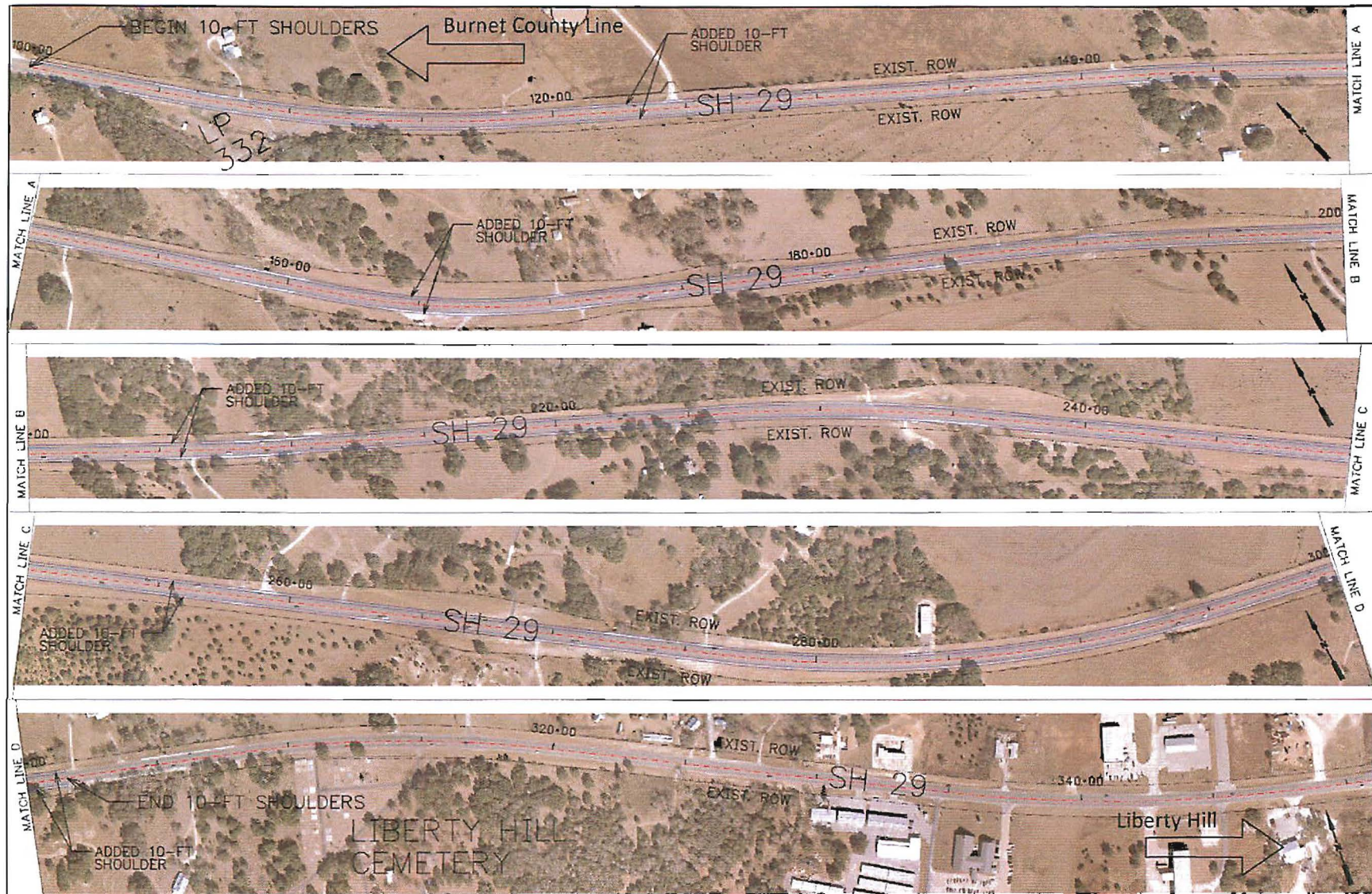
Figure 34. Burnet Co. Line to Liberty Hill Cemetery: 10-ft improved shoulders
