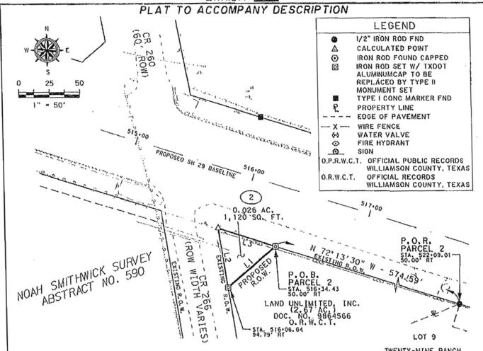
I) ALL BEARINGS ARE BASED ON GRID BEARINGS, DISTANCES ARE SURFACE DISTANCES. COORDINATES ARE SURFACE VALUES BASED ON THE TEXAS STATE PLANE COORDINATE SYSTEM, NAD 83, CENTRAL ZONE, USINO A COMBINED SURFACE ADJUSTMENT OF 1.00014
