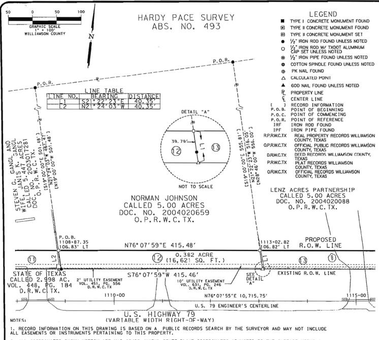
2. ALL COORDINATES SHOWN HEREON ARE NAD 83/93 (HARN) STATE PLANE COORDINATES ADJUSTED TO THE SURFACE USING A COMBINED SCALE FACTOR OF 1.0001135512.
