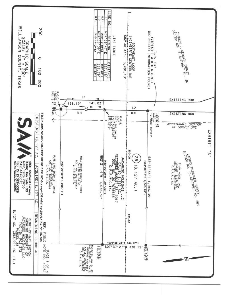
80D NAIL FOUND TXDOT TYPE II BRONZE DISK IN CONCRETE FOUND 5/8" IRON ROD SET WITH ALUMINUM CAP STAMPED "WILLIAMSON COUNTY" 1/2" IRON PIPE FOUND UNLESS NOTED TYPE I CONCRETE MONUMENT FOUND FENCE POST (TYPE NOTED) 1/2" IRON ROD FOUND UNLESS NOTED LEGEND EXHIBIT Α. 196.12 EXISTING ROW WILLIAMSON COUNTY, TEXAS
