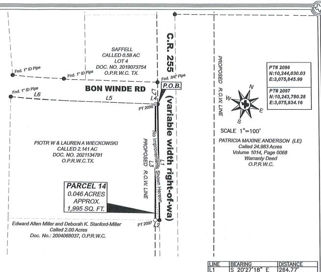
ALL BEARINGS, DISTANCES, COORDINATES AND AREAS ARE BASED ON THE TEXAS COORDINATE SYSTEM OF 1983 (NAD83), TEXAS CENTRAL ZONE, BASED ON GPS SOLUTIONS FROM THE NATIONAL GEO DETIC SURVEY (NGS) ON-LINE POSITIONING USER SERVICE (OPUS).
