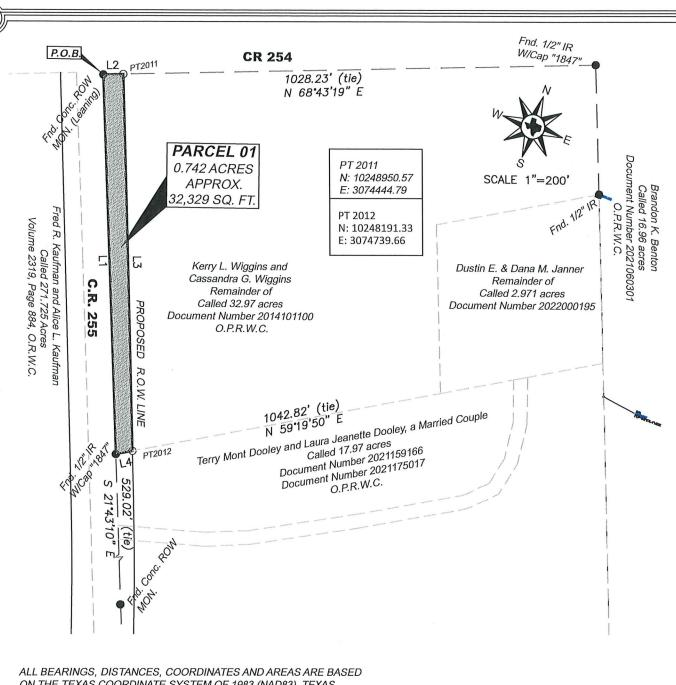
ALL BEARINGS, DISTANCES, COORDINATES AND AREAS ARE BASEL ON THE TEXAS COORDINATE SYSTEM OF 1983 (NAD83), TEXAS CENTRAL ZONE, BASED ON GPS SOLUTIONS FROM THE NATIONAL GEO DETIC SURVEY (NGS) ON-LINE POSITIONING USER SERVICE (OPUS).
