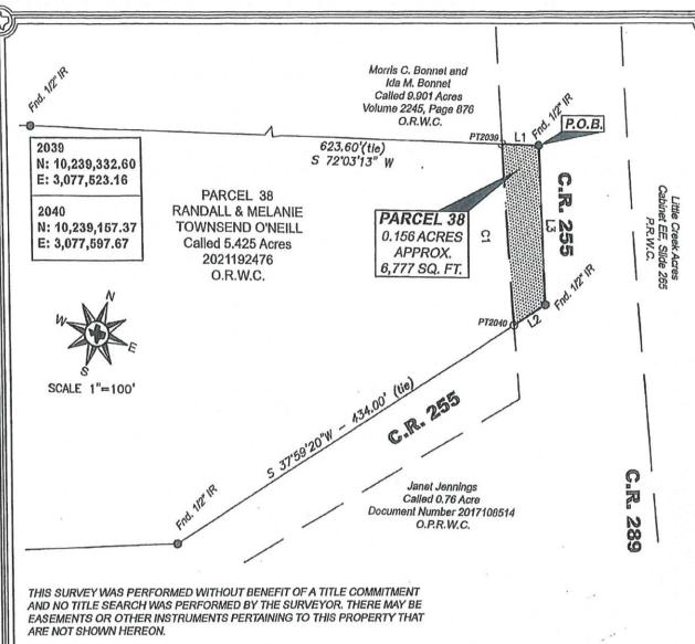
ALL BEARINGS, DISTANCES, COORDINATES AND AREAS ARE BASED ON THE TEXAS COORDINATE SYSTEM OF 1983 (NAD83), TEXAS CENTRAL ZONE, BASED ON GPS SOLUTIONS FROM THE NATIONAL GEO DETIC SURVEY (NGS) ON-LINE POSITIONING USER SERVICE (OPUS).
