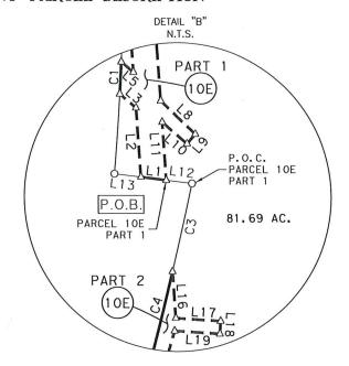
1) All bearings shown hereon are based on grid bearing. All distances are surface distances. Coordinates are surface values based on the Texas State Plane Coordinate System, NAD 83, Central Zone.
