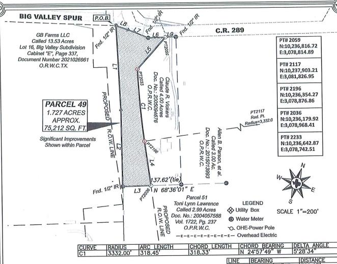
ALL BEARINGS, DISTANCES, COORDINATES AND AREAS ARE BASED ON THE TEXAS COORDINATE SYSTEM OF 1983 (NAD83), TEXAS CENTRAL ZONE, BASED ON GPS SOLUTIONS FROM THE NATIONAL GEO DETIC SURVEY (NGS) ON-LINE POSITIONING USER SERVICE (OPUS).
