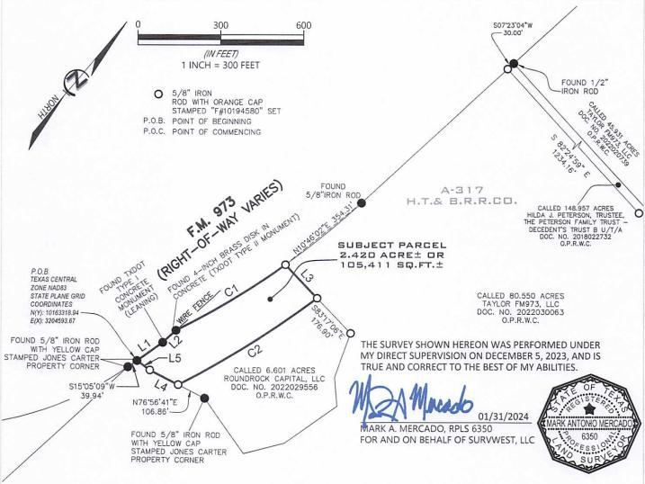
1.) DISTANCES ARE IN U.S. SURVEY FEET AND ARE DISPLAYED IN SURFACE VALUES USING A COMBINED AVERAGE SCALE FACTOR OF 1.000108 GENERATED FROM NATIONAL GEODETIC SURVEY (NGS) ONLINE POSITIONING USER SYSTEM (OPUS) SOLUTIONS.
