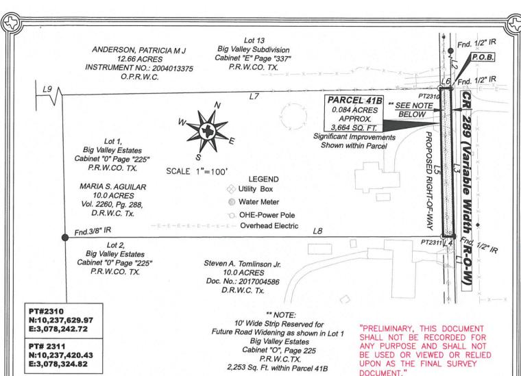
ALL BEARINGS, DISTANCES, COORDINATES AND AREAS ARE BASED ON THE TEXAS COORDINATE SYSTEM OF 1983 (NAD83), TEXAS CENTRAL ZONE, BASED ON GPS SOLUTIONS FROM THE NATIONAL GEO DETIC SURVEY (NGS) ON-LINE POSITIONING USER SERVICE (OPUS).
