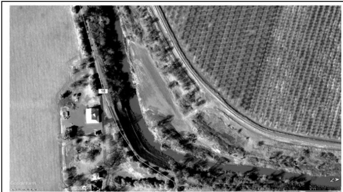
Figure 2. Aerial image of the Huff's Corner levee-stream system in February 2008, showing the recent removal of accumulated sediment in the upstream end of the widened zone. The widened zone functions to retain ('trap') sediments because of reduced stream power. Note retained 'island,' possibly intended to force flows to the left ('inside') streambank. North is to right.
