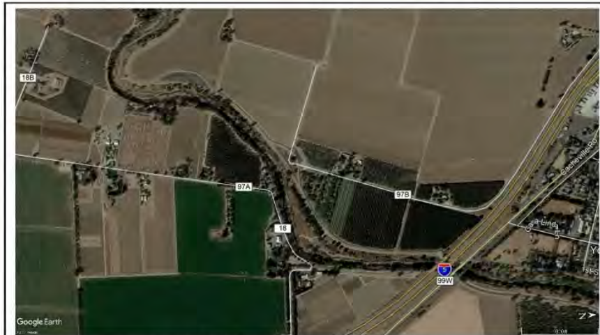
Figure 1. Regional image of the Cache Creek levee-channel system in the vicinity of the Huff's Corner project, October 2020. Note the relatively constant narrow width throughout the region and the wider zone between the levees in the project area (center of image). Flow and discharge within the channel system are continuous, and the widened zone allows flows to slow, reducing the stream's ability of transport sediment and resulting in its deposition. North is to right.
