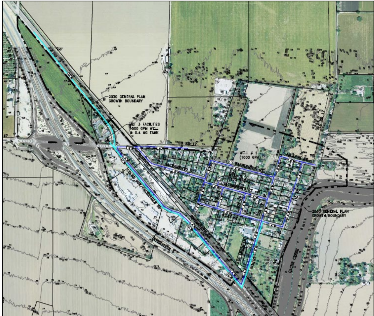
Figure 1. Proposed Water System Configuration – 2030 Buildout
