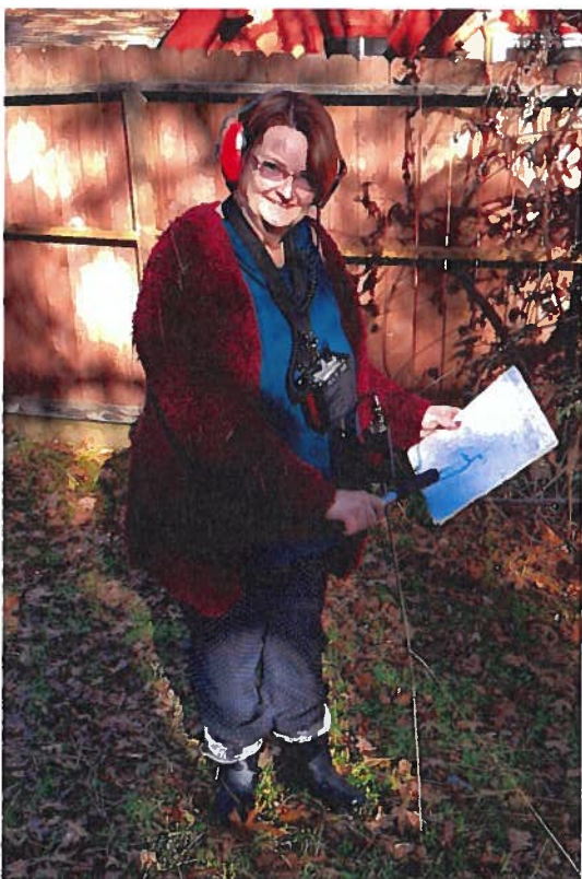
Angela using leak detection equipment and as-builts to narrow down leak location.
