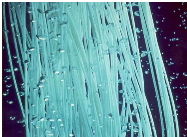
Figure 2. Hollow-fiber membranes (Image from GE/Zenon)
