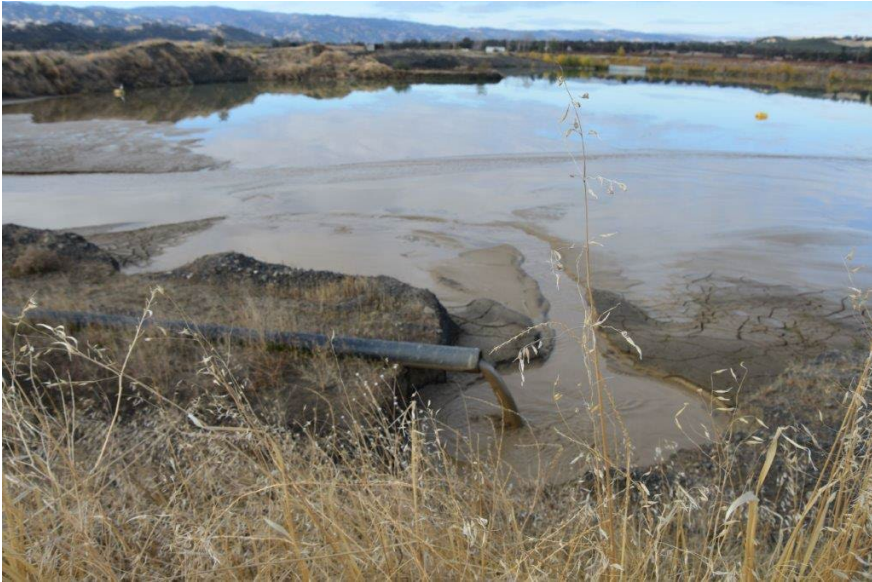
Wash Fines Pumped into Pit for Future Reclamation
