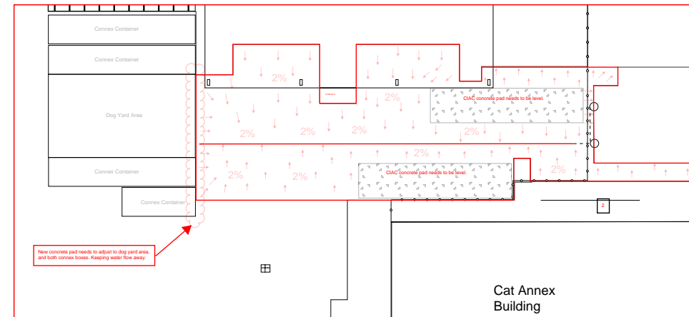
Concrete Slab Slope
